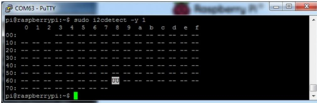
A terminal window titled 'COM63 - PuTTY' showing the output of the command 'sudo i2cdetect -y 1'. The output is a grid of dashes representing I2C addresses, with 'UU' appearing at address 60, indicating a hardware clock is present.
